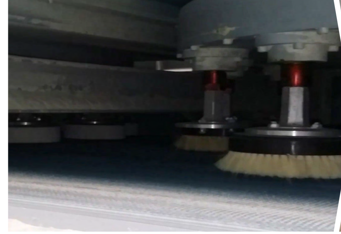
Spazzole in movimento Working brushing tools
